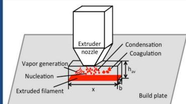
Fig.2 Schematic of the control volume and aerosol dynamic processes that are modeled within the control volume
