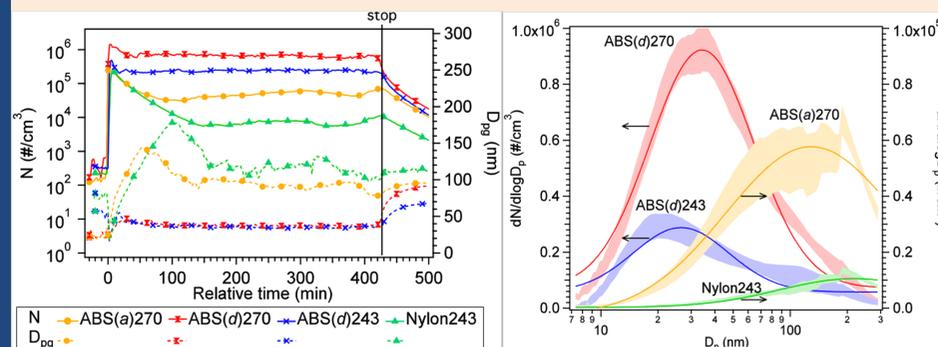
Fig.3 Total particle number concentrations and geometric mean diameters measured in chamber
