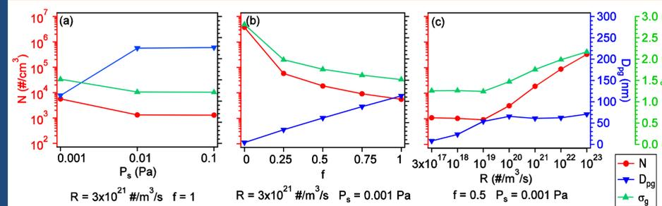
Fig.5 The simulated steady state particle characteristics (N,  $D_{pg}$ ,  $\sigma_g$ ) as a function of each vapor property ( $P_s$ , f, R) separately when controlling the other two
