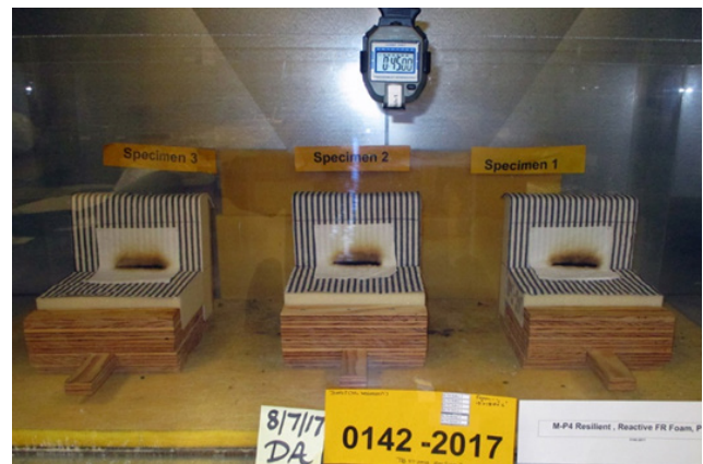
California Technical Bulletin 117-2013 (TB 117-2013) smolder resistance test in triplicate.
