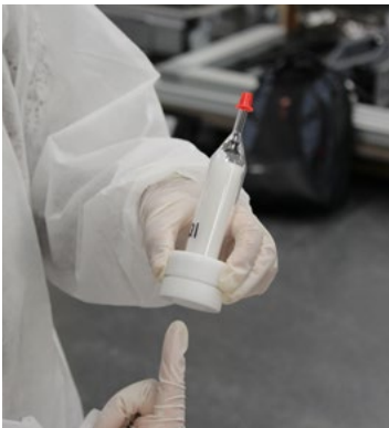
Figure 9: Environmental exposure sampling media for airborne flame retardants.
