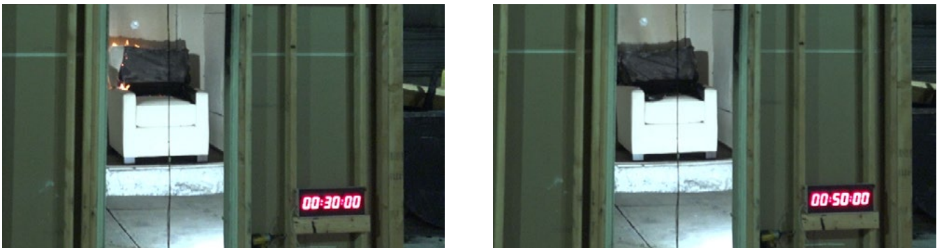
Figure 24: Still frames of the ISO 9705 Test Room burns for no flame retardant with barrier textile (BNFR) chair at 30 and 50 minutes from ignition.
