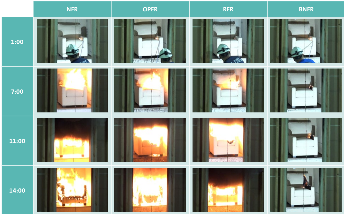
Figure 23: Still frames of the ISO 9705 Test Room burns for no flame retardant (NFR), organophosphate flame retardant (OPFR), reactive flame retardant (RFR), and no flame retardant with barrier textile (BNFR) chairs at 1, 7, 11, 14 minutes from ignition.
