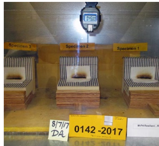
Figure 15: California Technical Bulletin 117-2013 (TB 117-2013) smolder resistance test (typical) showing testing of reactive flame retardant polyurethane foam.
