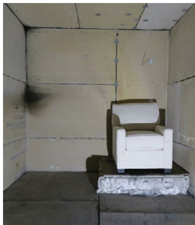
Figure 14: An ISO 9705 Test Room setup (left) with a chair on a corner load cell assembly (right).
