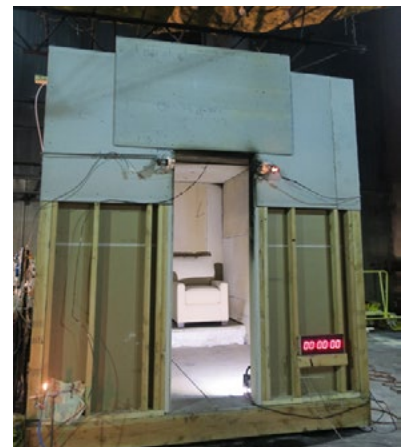
Figure 14: An ISO 9705 Test Room setup (left) with a chair on a corner load cell assembly (right).
