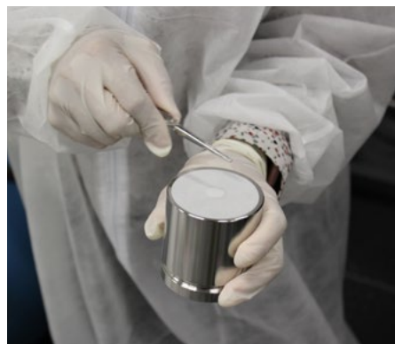
Figure 11: Dermal transfer sample collection from chair (left) shows the filter patch ready to be placed on a chair (right).
