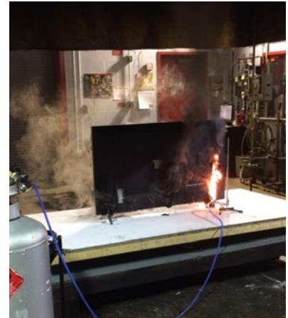
Figure 13: Furniture Heat Release Calorimeter open room setup with a chair (left) and a television (right) on the load cell assembly.
