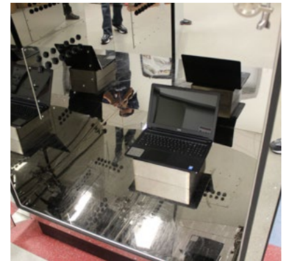
Figure 5: Chair (left) and electronic test products (laptop on right) in an environmental chamber.
