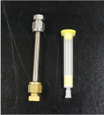
Figure 8: Environmental exposure sampling media for air sampling: Tenax® tube (left) and 2,4-dinitrophenylhydrazine (DNPH) cartridge (right) for volatile organic compounds (VOCs) and aldehydes respectively.
