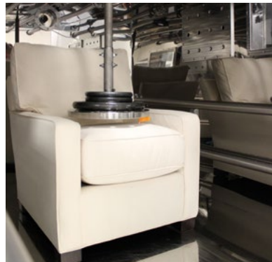
Figure 5: Chair (left) and electronic test products (laptop on right) in an environmental chamber.
