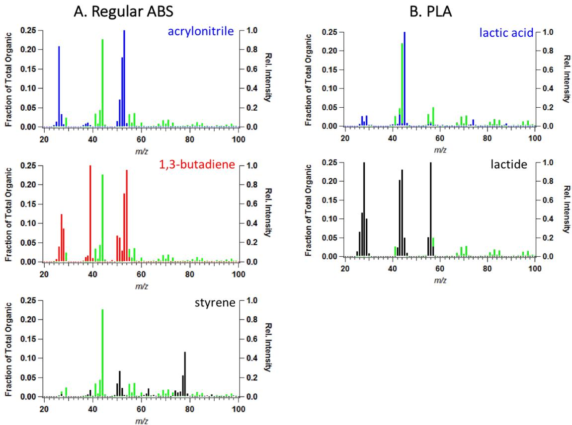
Figure 1. Particle mass spectra measured by ACSM (shown in green) of particles emitted from Regular ABS (A) and PLA (B). Reference spectra of monomers corresponding to the raw filament materials for ABS (acrylonitrile, blue; 1,3-butadiene, red; styrene, black) and PLA (lactic acid, blue; lactide, black) are included for comparison.<sup>12</sup>
