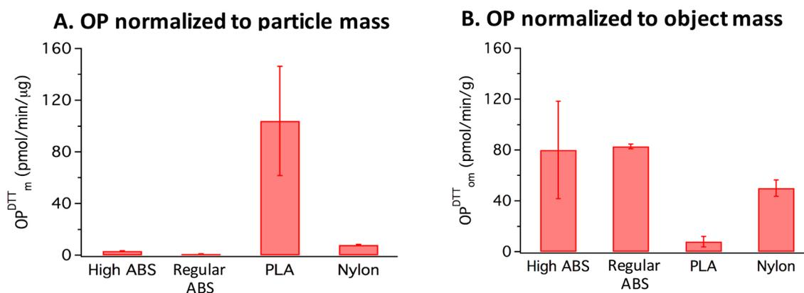
Figure 4. Total DTT assay results presented as OP normalized to particle mass (A) or OP normalized to print object mass (B). The difference between the two is whether particle emission levels were considered.
