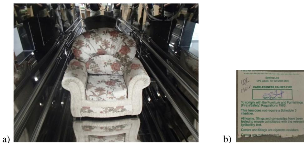
Figure 1: a) U.K. chair in a chamber b) a tag attached to the chair
