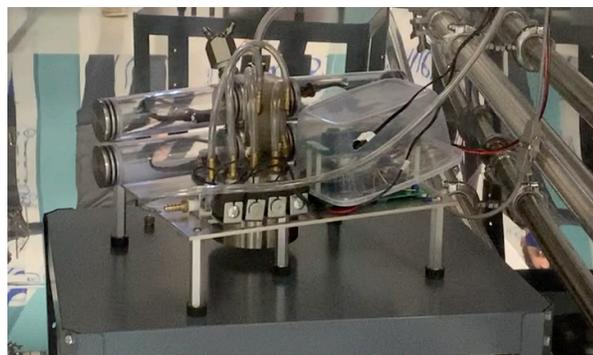
The ENDS aerosol generator is shown above in the environmental exposure chamber.
