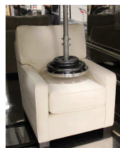
Figure 1: A studied chair inside an environmental exposure chamber with a device to mimic a person sitting.
