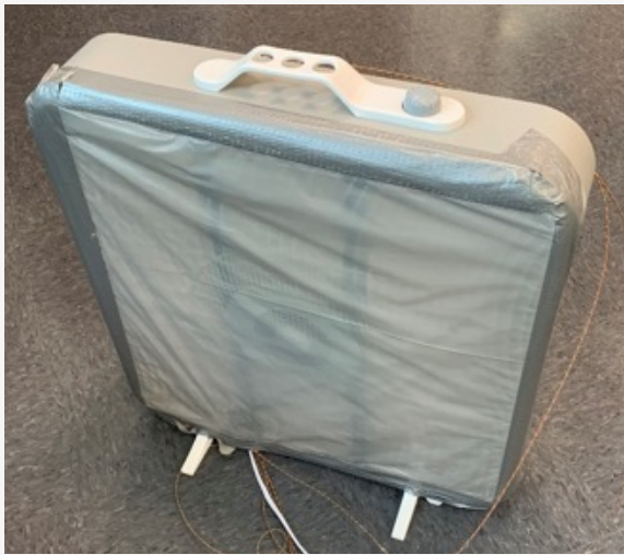
Figure 3: Pictures of the tested box fans with thermocouples attached, one side blocked (left) and both side blocked when lying face down (right).
