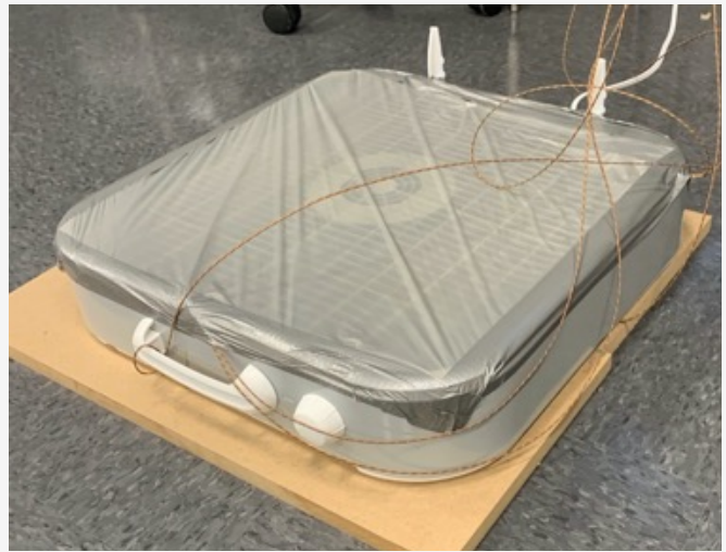
Figure 3: Pictures of the tested box fans with thermocouples attached, one side blocked (left) and both side blocked when lying face down (right).
