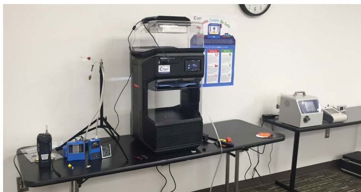
Figure 4: A room with instruments: A PID, pumps with sampling media, a 3D printer with cassette filter attached, and a SMPS (from left to right).
