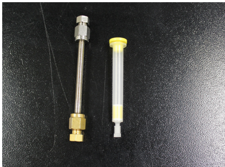
Environmental exposure sampling media for air sampling: Tenax® tube (left) and 2,4-dinitrophenylhydrazine (DNPH) cartridge (right) for volatile organic compounds (VOCs) and aldehydes respectively.
