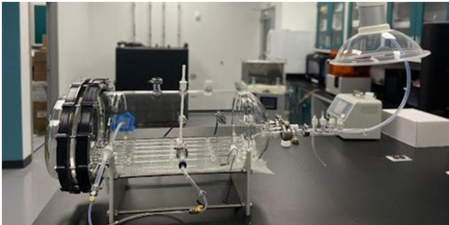
Figure 1: Glass chamber set up. Clean air entering the chamber on the left, vape pen operating in the middle on the glass rack, and air samples collected downstream to the right of the chamber.
