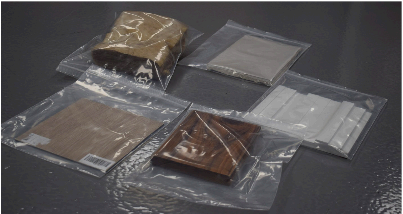
Figure 1: The five building materials for the study. Clockwise from the top right: drywall, MDF, engineered wood flooring, vinyl flooring and batted fiberglass insulation.
