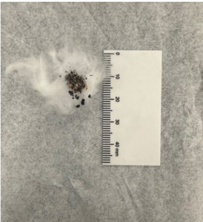
Figure 1: Dust sample on quartz wool prior to testing.
