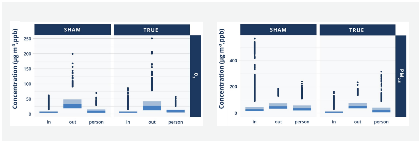
Figure 3: Summary of hour-averaged PM 2.5 and ozone concentrations for all homes in the Shanghai study. These data collected using low-cost monitors illustrate the higher concentrations of PM 2.5 and ozone outdoors as compared to indoors and highlight the benefit of filtration for PM 2.5 indoors and, to a lesser extent, for personal exposure to PM 2.5 . 3
