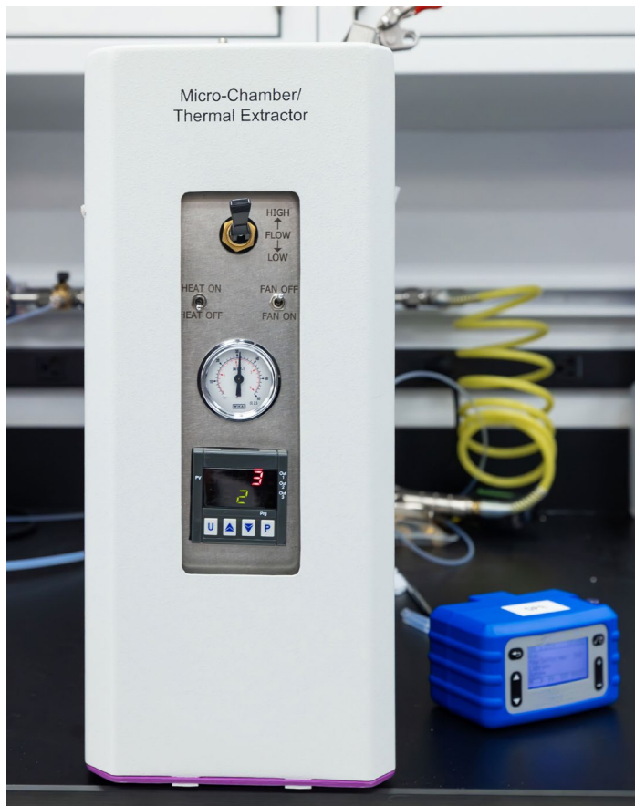
Figure 1: A microchamber equipped with a heating device and humidity apparatus.
