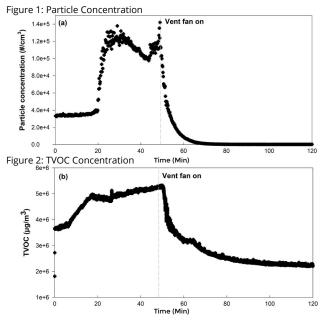
Figures 1 and 2 show a significant drop off in particle and TVOC emissions after a vent fan is turned on. **Credit: NIOSH.**
