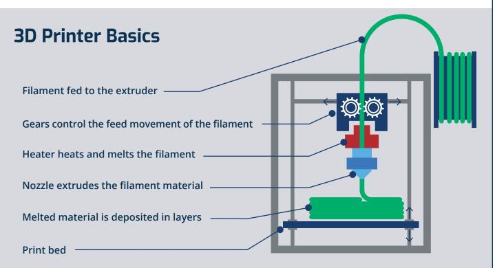
Fundamentally, 3D printers take a digital file and use it to build a three-dimensional solid object. The most common consumer-level 3D printers use a method called fused filament fabrication, or FFF. That simply means that the printer heats up a material, forces it through a nozzle, and then deposits – or prints – that material layer by layer to build an object.
