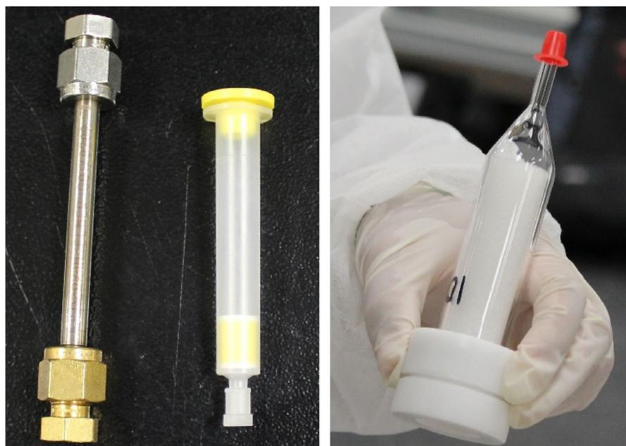
**FIGURE 4** Environmental exposure sampling media for air sampling: Tenax® tube (left) and 2,4-dinitrophenylhydrazine (DNPH) cartridge (middle) for volatile organic compounds (VOCs) and aldehydes respectively, and quartz filter in line with PUF cartridge for airborne FR (right)
