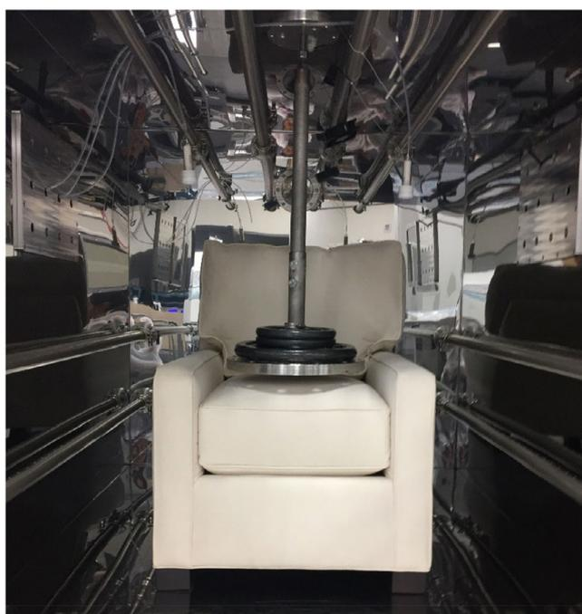
FIGURE 2 Chair and the automated sitting mechanism in an exposure chamber
